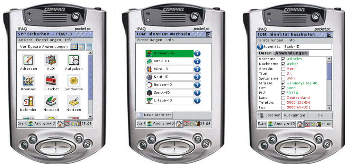
Figure 5-6: Integration of the iManager in the user interface of the mobile device
